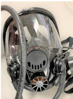
Some may think it total overkill, but the Navy insists that everyone: (the Chemist, the workers opening the tank, and the safety watch at the enclosure opening) must have a full-face supplied air protection for any opening of a sewage system. What a pain! But in this case the "pain" turned out just basic baseline safety. Supplied air was the go-to minimum protection for an IDLH situation. (Continued)
